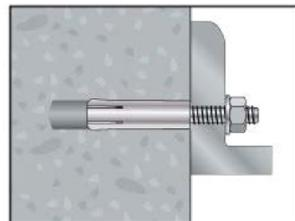
5. To fix the fixture, not allowed to pass over the max. installation torque  $T_{inst}$
