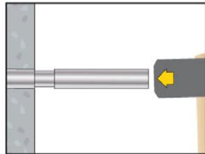
4. To spread the anchor with the setting tool. The anchor is installed correctly, if the setting pin is completely inside
