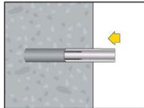
3. To set the anchor by hand or by hammer blows, anchor should be flush to the concrete edge
