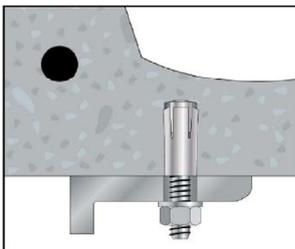
5. Installed SA in precast prestressed hollow core slab
